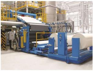
membranes rolls have a net width of 2000 mm and a thickness up to 2000  $\mu.$  The output is 2.000 Kg/h.
