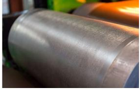
AMUT unique solution for post-embossing of the edgebanding surface has been upgraded and today it allows the changeover of embossing pattern in few seconds without any production loss or extrusion speed reduction.
