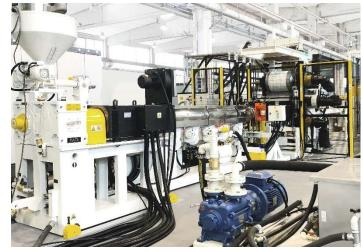
Thanks to a special double venting screw design it is possible to reach perfect quality product with no extra costs and low energy consumption. The extruder has a 52L/D ratio and can process as well the latest PP edgebanding.
